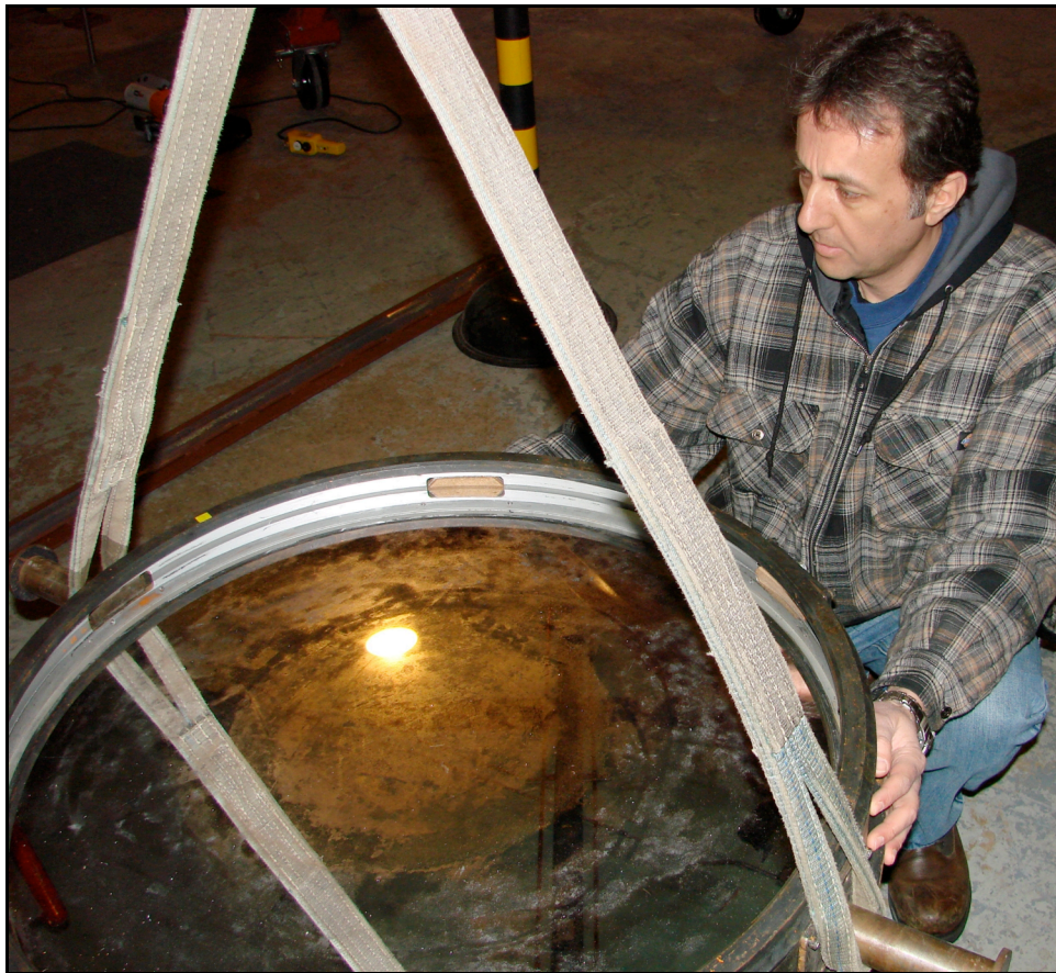
Kostas Chloros examining the 120" Coude' secondary with its severely degraded coating.
