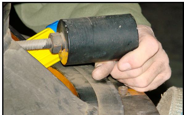
Support the weights with your hand while loosening the suspension bolts
