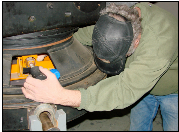
Set the mirror onto the wooden flipping frame. Unscrew the three suspension bolts from the back of the glass.
